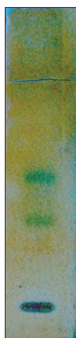
Figure 3: TLC of leaf ethanolic extract in visible light after spraying with Dragendorff reagent
