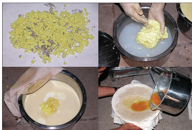
Figure 2: Steps involved in purification of sulfur
