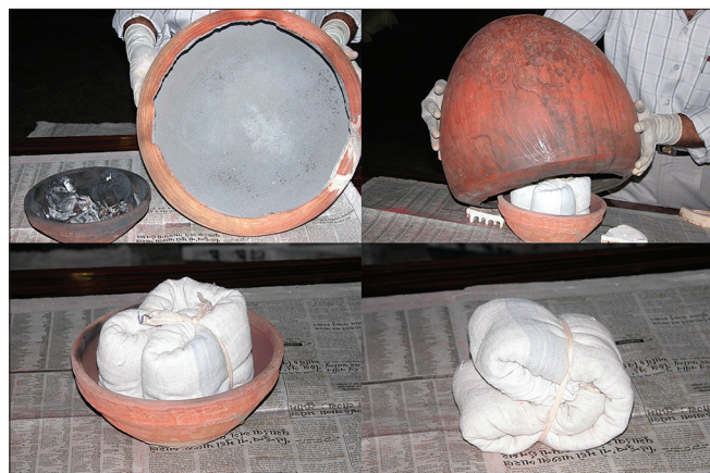
Figure 3: Steps involved in extraction of mercury from cinnabar
