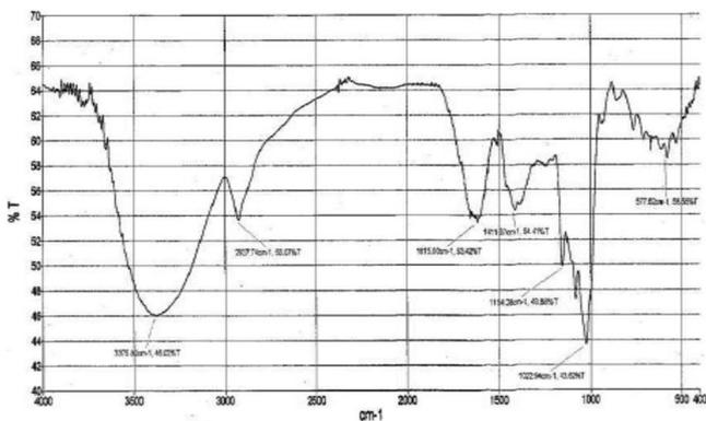
**Fig. 5. FTIR analysis.** The figure represents the FTIR spectra of the  $\beta$ -ecdysone containing peak of the *T. cordifolia* extract showing the hydroxyl absorption at  $\sim 3500$  cm and carbonyl absorption at  $\sim 1645$  cm as compared to the reference spectrum of  $\beta$ -ecdysone retrieved from spectral library.
