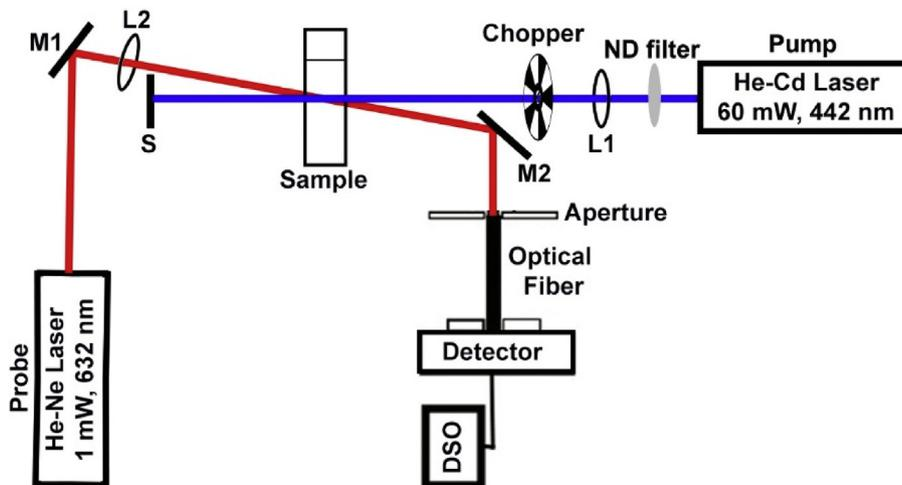
Fig. 1. Schematic diagram of mode-mismatched dual-beam thermal lens technique.
