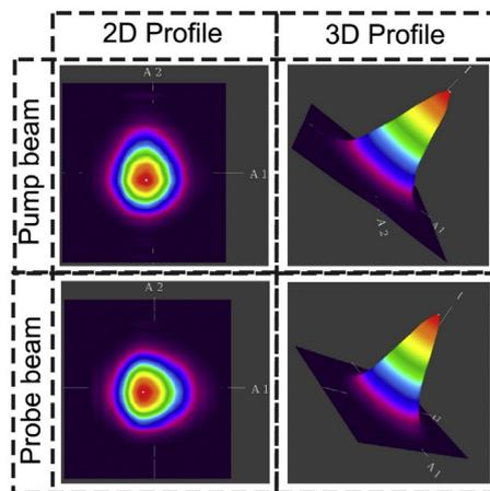
Fig. 2. 2D and 3D profile of the pump and probe beam.
