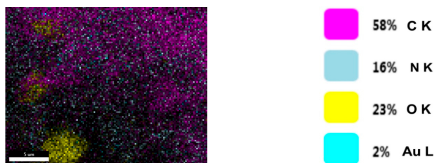
Figure 9. Engineered viscum–AuNPs carrier assembly: SEM—live map.
